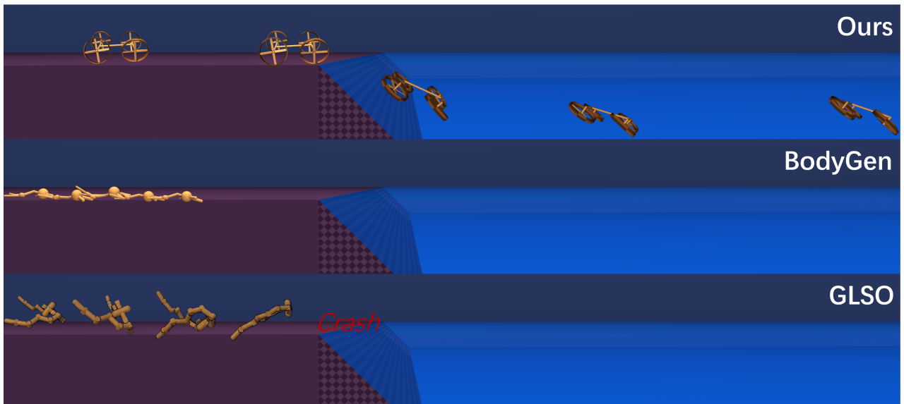
Figure 20. Visualization of comparison with morphology-co-design baselines of Wheel-fly (swim) experiment, containing four frames in T = 8, 11, 14, 17, 20 s respectively. “Crash” means the algorithm makes the robot crash at this point.
