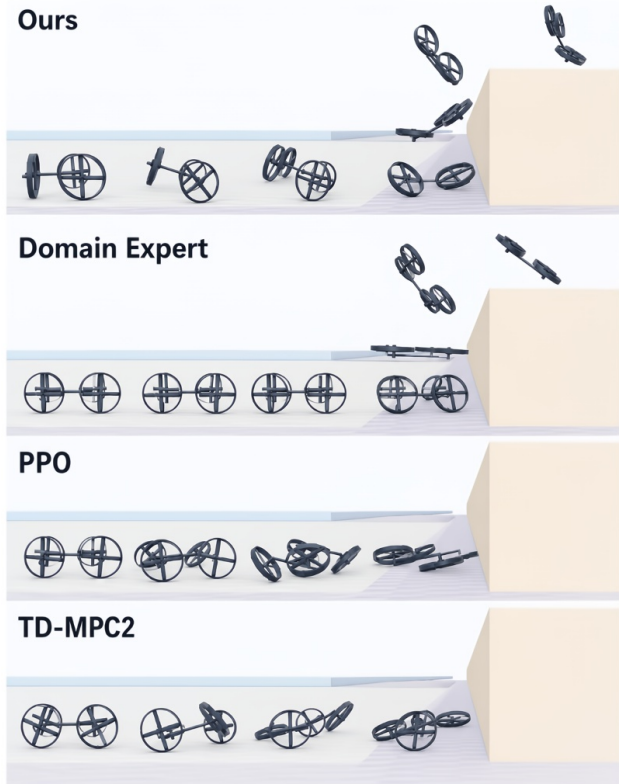
Figure 3. Visualization of the comparison among our pipeline, Domain-expert, PPO, and TD-MPC2 on wheel-fly (mount) task. PPO and TD-MPC2 are all stuck at the bottom of the mountain. While domain-expert successfully fly over the mountain, our pipeline demonstrate higher performance.
